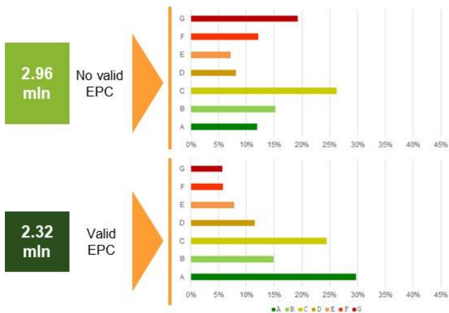
Diagram: Overview of (estimated) energy label distribution of the Dutch property stock.
